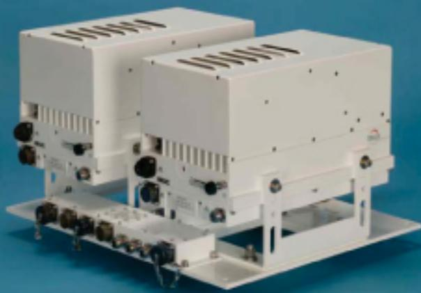
The integration of 1+1 protection was a key design goal in Terrasat's IBUC Intelligent Block Upconverters development. The IBUC redefines 1+1 protection switching. Instead of using a separate switching logic unit with its expense and complexity, Terrasat incorporated the switching logic and drivers into the IBUC itself.
