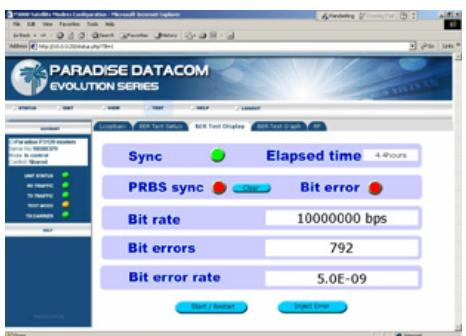
**Unique Web User Interface provides full Monitor & Control plus graphing of Eb/No, BER, Receive Power and other operating parameters, plus a Receive Spectrum Analyser, Receive Constellation Monitor and BER Tester for detailed signal analysis and performance validation via Internet Explorer. Logged graph data can be sent via email to any email address.**
