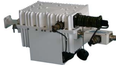
Figure 3: DC blocked to IF port (Options “F” and “P”)
