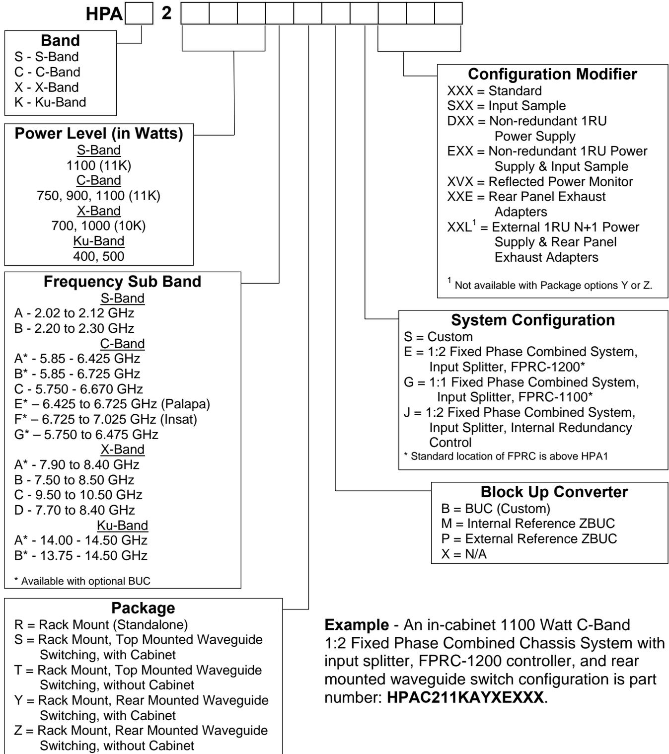
**Example** - An in-cabinet 1100 Watt C-Band 1:2 Fixed Phase Combined Chassis System with input splitter, FPRC-1200 controller, and rear mounted waveguide switch configuration is part number: **HPAC211KAYEXXX**.
