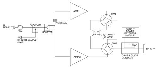
1:1 Phase Combined System Simplified Block Diagram
