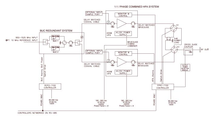
The Block Up Converter system is housed in a 1RU rack-mountable enclosure and controlled by a RCP2-1100 Redundant Controller. The Up Converters can be configured with internal reference oscillators or external reference oscillators. The Paradise Datacom ZBUC architecture allows a converter that is fitted with an internal reference oscillator to automatically detect and switch to an externally applied 10 MHz reference signal.
