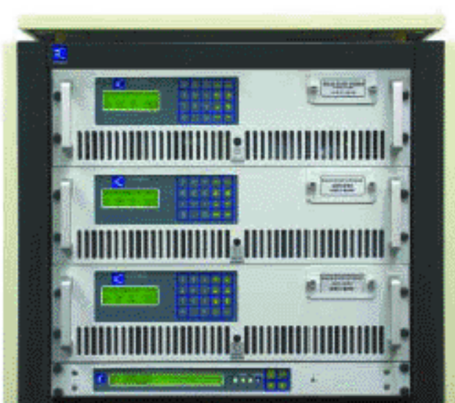
Front view of 1:2 SSPA redundancy system
