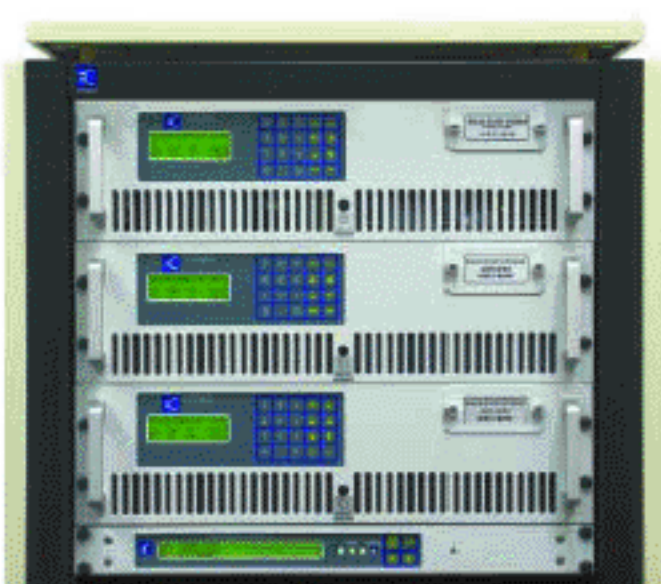
Front view of 1:2 SSPA redundancy system
