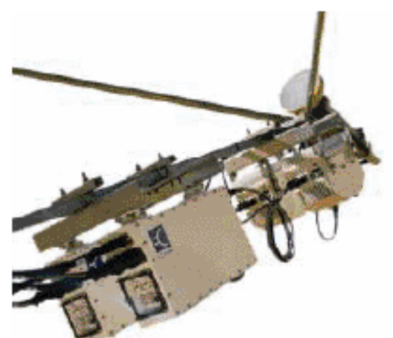
5700 transceivers antenna mounted in 1:1 configuration
